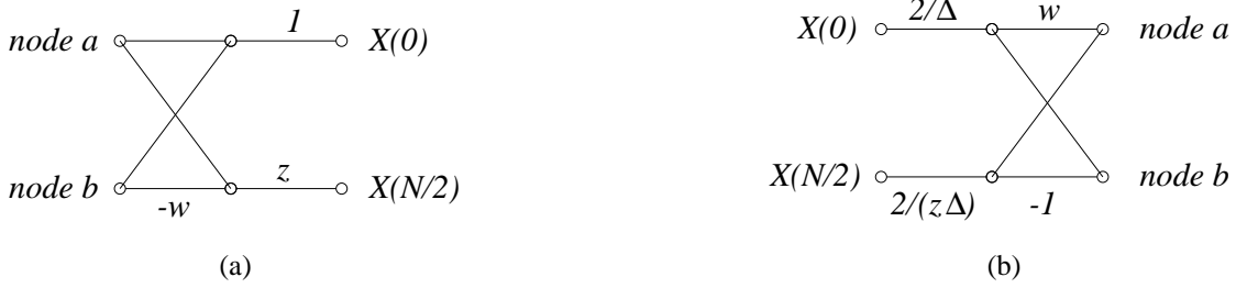
Fig. 6. (a) Modification of butterflies in the flowgraph from Fig. 3 leading to the orthogonalization of basis functions. (b) Non-normalized inverse butterfly for butterfly from (a).
